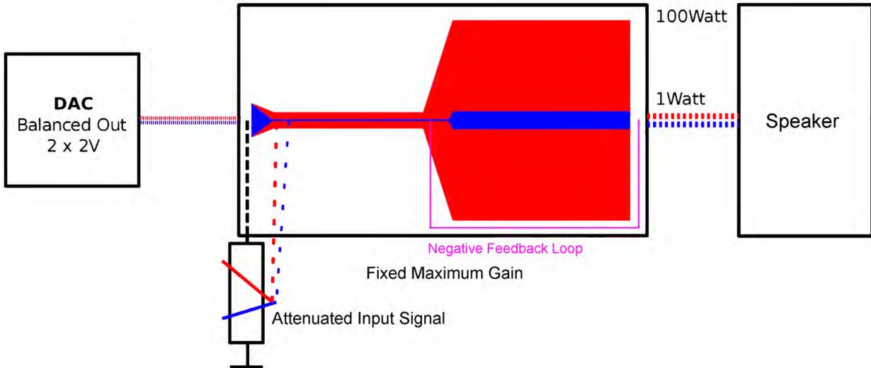
**Red** = High volume: The input signal is reduced from 4V to less than 1V, then amplified about 30 times.
