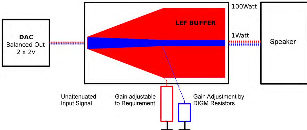
**Red** = High volume: The unattenuated input signal of 4V is amplified about 7 times.
