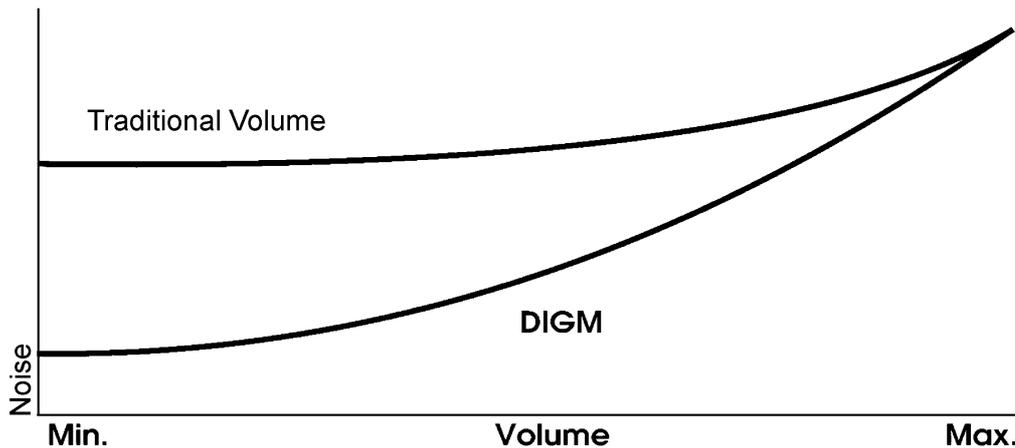
With the integrated B.M.C AMP volume adjustment through the DIGM circuit can either be triggered by the remote control or the volume control on the front panel. With the B.M.C. power amplifiers volume adjustment is triggered through an optical connection to the DAC1, use the remote control of the DAC1 or the volume control on its front panel.
